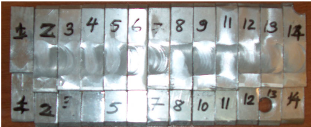
Fig. 5 Tensile shearing test samples machined out from FSW lap joints. All of the FSW lap joints were obtained with 1200 rpm tool rotation and 60 mm/min traverse speed (samples numbered 1, 2, 3, and 4 are from AA 2014 + AA 2014; samples numbered 5, 6, 7, 8, and 9 are from AA 6063 + AA 6063 and samples numbered 11, 12, 13, and 14 are from AA 6063 + AA 2014 combinations)
